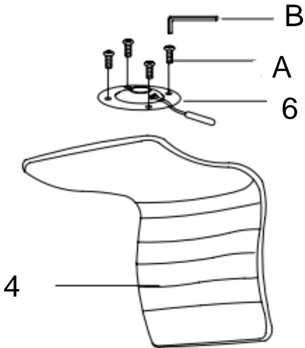
Attach bracket w/handle (6) to seat (4) by using bolt (A) and wrench (B) as shown.
