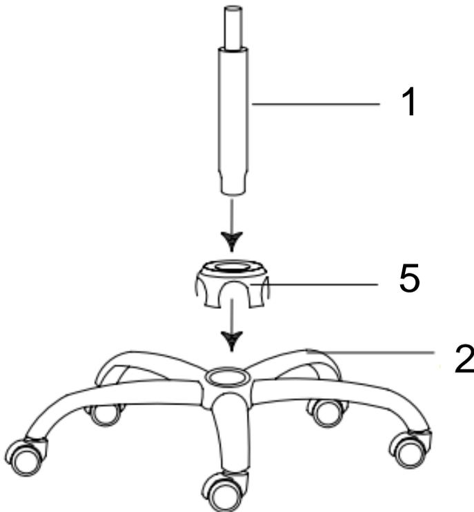
Insert base cap (5) and gas lift (1) into base (2) carefully as shown.
