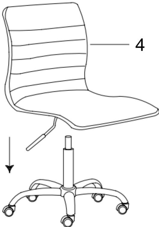
Insert gas lift (1) into seat (4) by applying moderate downwards force to the seat (4) in order to secure it to the base as shown.
